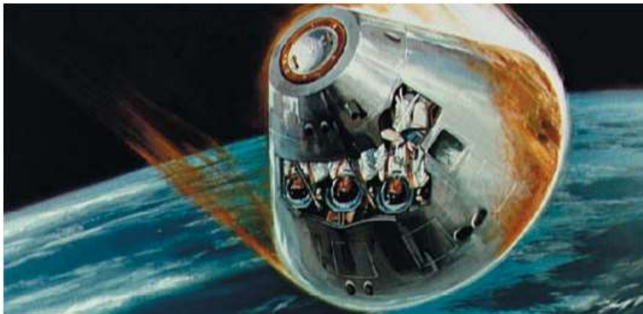
Figure 4.1.7-1. Apollo Capsule Re-entry. This artist's concept of the Apollo re-entry shows that air friction causes the capsule to glow red hot. The astronauts inside stay cool, thanks to the protective heat shield. (Courtesy of NASA/Johnson Space Center)
